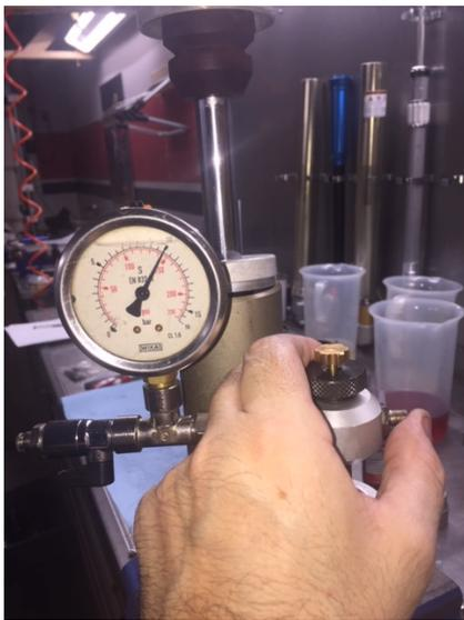
**TOGLIERE LA PRESSIONE IN ECCESSO TRAMITE LA VALVOLA LATERALE, SPINGENDO CON UN DITO.**
