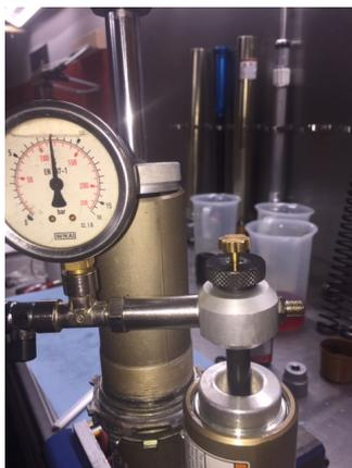
**UNA VOLTA RAGGIUNTO LA PRESSIONE VOLUTA, SVITARE IL POMELLO ORO E PORTARE LA PRESSIONE NEL MANOMETRO A ZERO TRAMITE LA VALVOLA LATERALE.**
