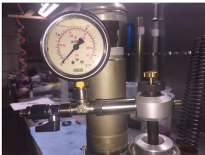
AVVITARE IL PRESSURIZZATORE NELLA VALVOLA SCHRADER E APPOGGIARE APPENA UN PO' LA GOMMA DI TENUTA INTERNA. ACCERTARSI CHE IL POMELLO ORO SIA TUTTO APERTO. METTERE A PACCO L'AMMORTIZZATORE COME IN FOTO
