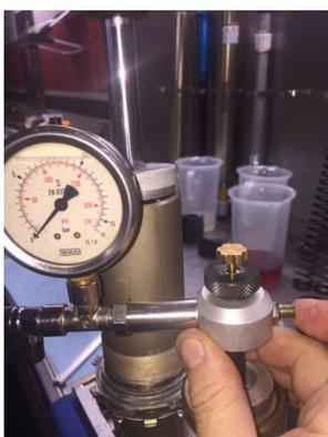
**UNA VOLTA CHE LA PRESSIONE E' A ZERO, E' POSSIBILE DISCONNETTERE TUTTO IL PRESSURIZZATORE DALLA VALVOLA.**
